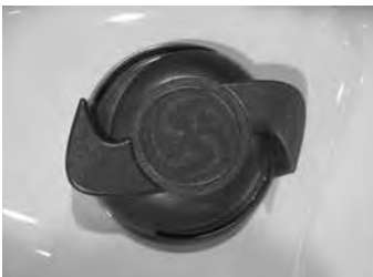
Air Control Valve
